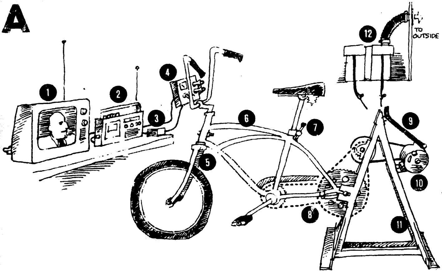
The prototype described here was built by the North Shore Ecology Center to find correct gear ratios for electric generation and for other foot-power mechanical devices. Possible applications might be: garden mulcher, flexible shaft drill, grinder, circular saw, air or water pump, etc.
